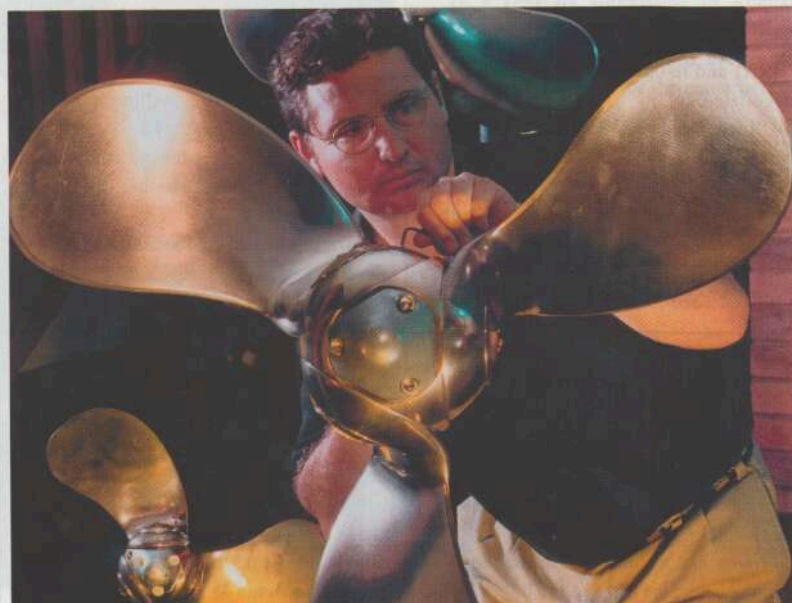
The automatic variable pitch propeller
