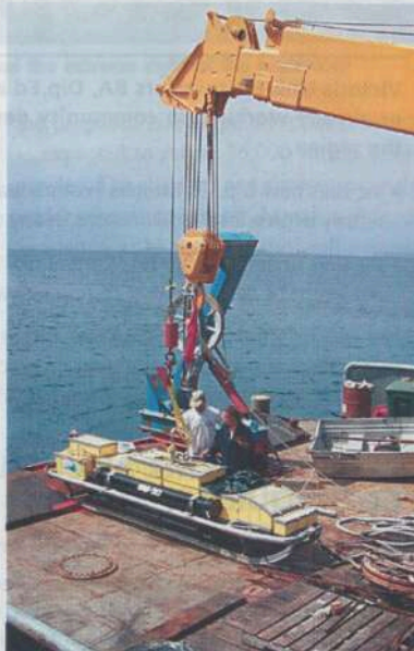
The high-tech "tow-fish" that will attempt to locate Earhart's plane using sonar
