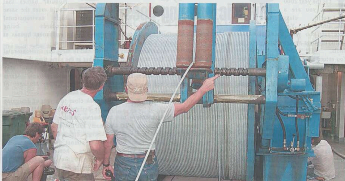
A reel holding 10,000 meters of heavy duty cable will hold a sonar-equipped "tow-fish" for the deep ocean search for Earhart's plane
