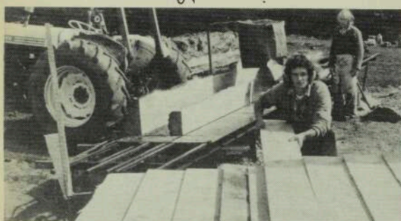
TRACTOR POWERED "VILLAGE" SAWMILL
