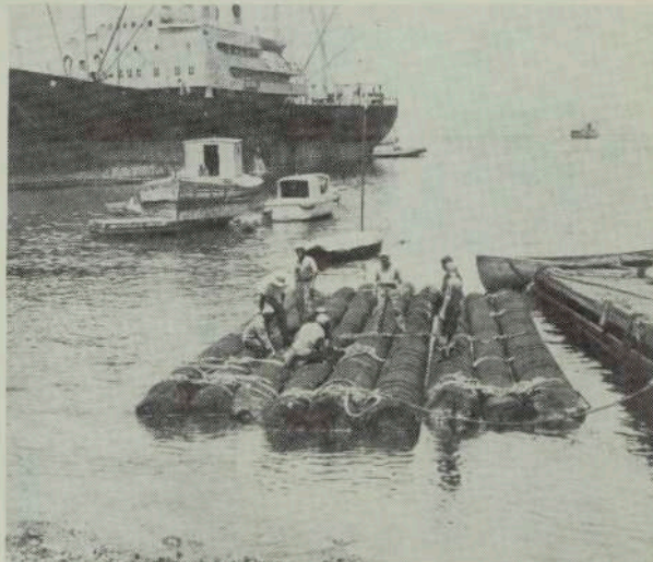
Peru, 1947, and the start of the adventure. Nine big balsa logs are lashed together to form the hull of the Kon-Tiki . (Picture from Thor Heyerdahl's book of the voyage). Opposite page: the Kon-Tiki on display today in Norway. Below: At sea in 1947. (Pictures from Mittet, Norway).
