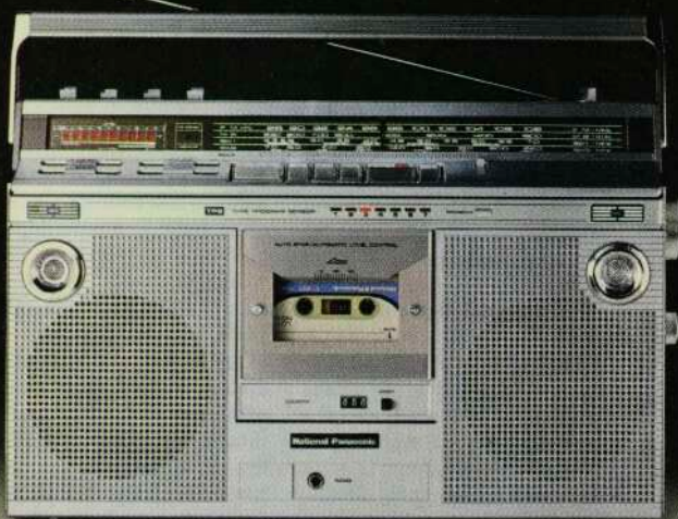
The RX-5300F has 12 watts output power and 4 bands: (FM/MW/SW 1 /SW 2 )
