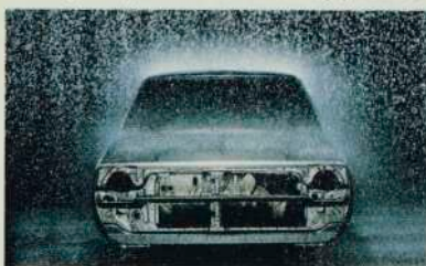
Special shower tests on a "white body."
