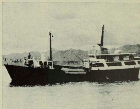
"M.V. Kaunitoni" - An Inter-Island freighter. Operated by the Fiji Government. Overall length 134.3 ft. Displacement 628 tons. Speed 10 knots. Powered by a Caterpillar D379.
