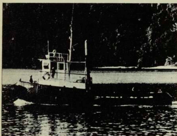
"Loloho" - General purpose Harbour tug boat. Operated by Bougainville Copper Limited at Bougainville. Overall length 50 ft. (15.24m). Powered by a Caterpillar D343 Marine Engine.
