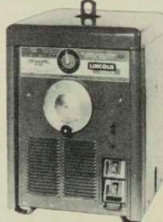
Lincoln TM heavy duty transformer and transformer/rectifier welders—range of six models for AC and AC/DC welding up to 750 amp, handling electrodes in the range 2.5 to 10 mm ( \frac{1}{8} " to \frac{3}{8} ") for all models. Input power 415 V 50 Hz single phase. Special voltages can be supplied.
