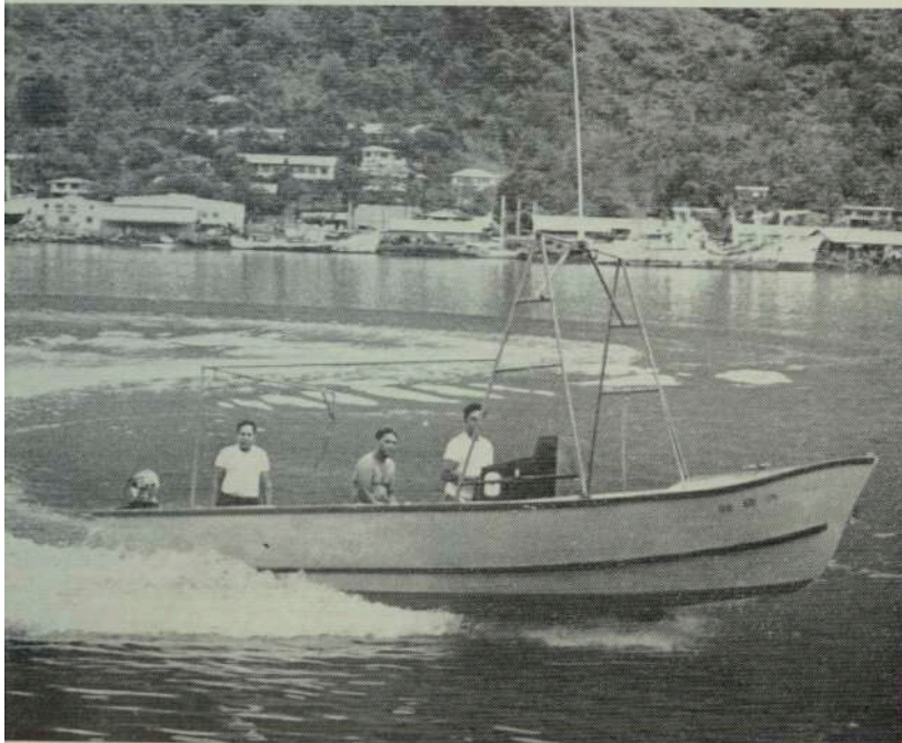
One of the new fast, trim dories being used in American Samoa for commercial fishing. Their design and the technique for their use come from Oregon, USA, and a team from that State has been helping to establish an industry based on them among Samoans.
