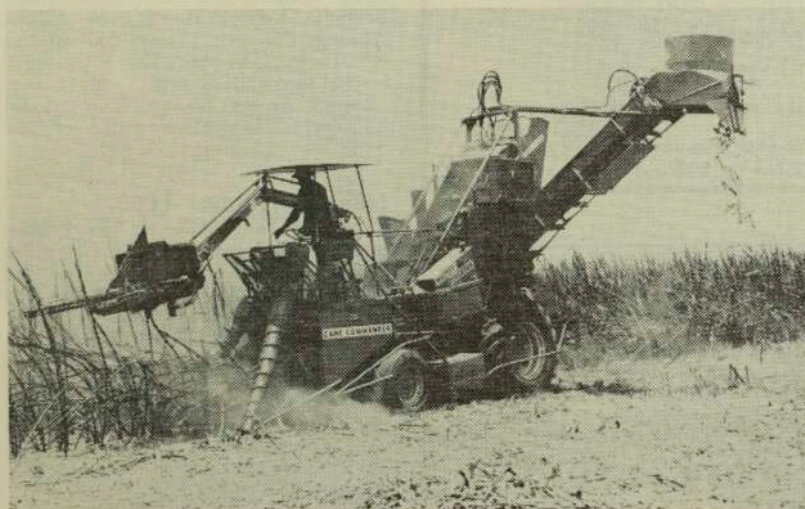
Tops fly and a steady stream of chopped cane is delivered from the spout as the Cane Commander gets into a heavier patch of the crop.
