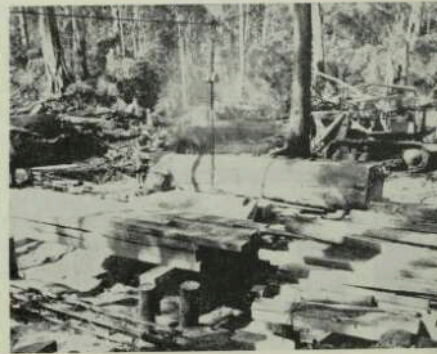
Cut flitches in the foreground. Note overhead chain bit with grabs for removing cut flitches from the log.
