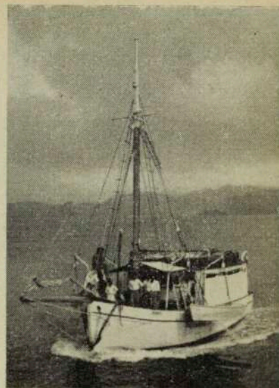
The 42 ft. long auxiliary ketch "Asha", recently fitted with a new 5 L.W. Gardner, at Lila and Sons boatyard, Suva, Fiji. Her reduction gear gives her a top speed of 13 knots and the owner now claims her to be the fastest vessel of her size in Fiji waters. Photo was taken at her engine trials in Suva. She will shortly go back into coastal service in the Group.
