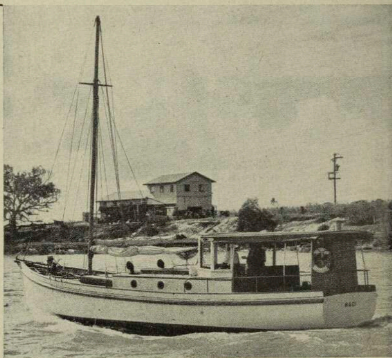
"MAGI" Recently delivered to Port Moresby. Our Standard 45 ft. Powered 6 L.W. 72 H.P. Gardner Diesel.
