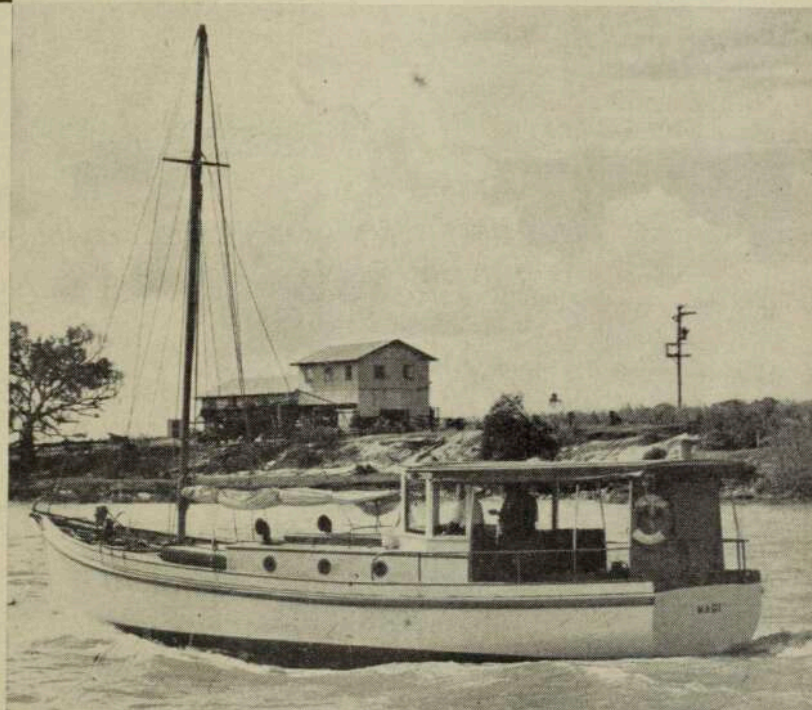
"MAGI" Recently delivered to Port Moresby. Our Standard 45 ft. Powered 6 L.W. 72 H.P. Gardner Diesel.
