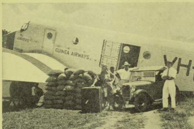
One of Guinea Airways' giant freight-carrying aeroplanes with a typical load. This big G-31 Junkers machine transported from Lae, on the coast, to Wau, the Goldfields centre in the interior, a Baby Austin motor car, an office safe, and 38 bags of rice—a total weight of nearly 2½ tons!
