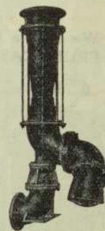
Hydraulic Elevator, with Swivelling Suction Pipe.
