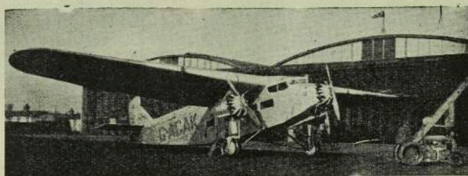
One of the new Ford Passenger 'Planes, the latest addition to our air fleet. The machine accommodates 10 passengers comfortably
