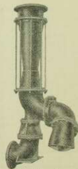
Hydraulic Elevator, with Swivelling Suction Pipe.
